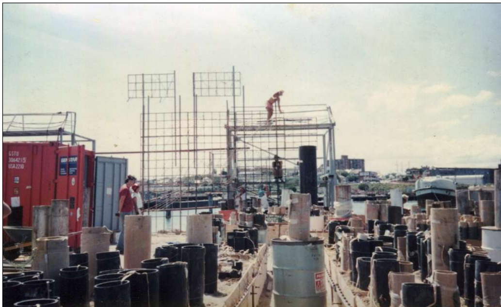
Preparing for the Bicentennial Fireworks. The set piece formwork can be seen at the rear. The mortars have been packed in sand on the barges. The shed to the left is where the pyrotechnicians sat to fire the shells.
